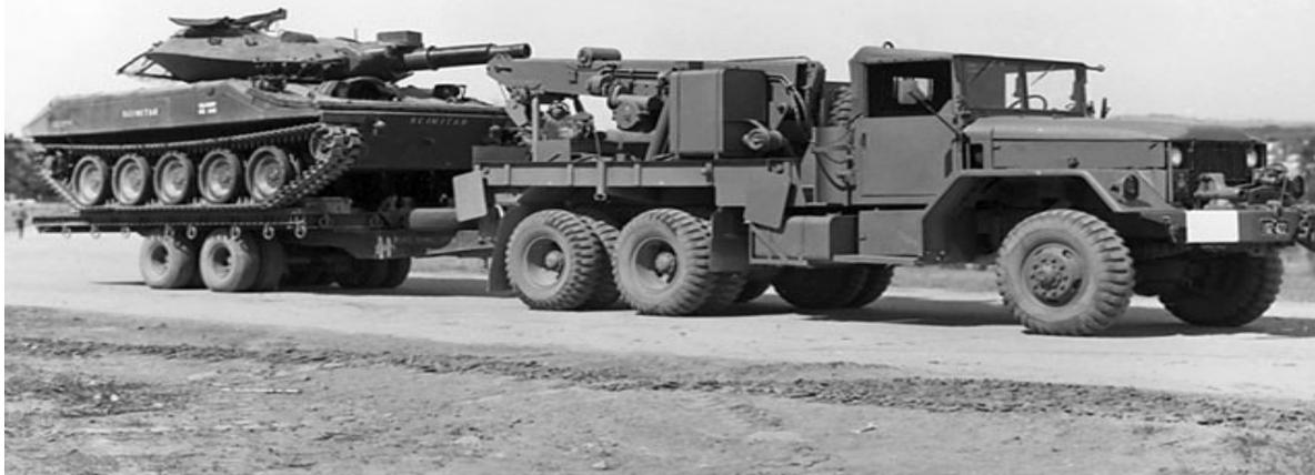
The Sheridan named Scimitar being carried on board an Australian Army 15 ton Tilt Bed Recovery trailer, and being towed by an M543 Wrecker. The Sheridan overhangs the deck of the trailer about half a track width on each side, making transport by that means very problematical.
