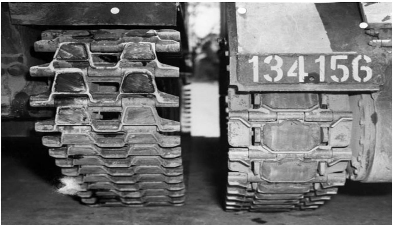
**Comparison of the track types of the Sheridan, left, and the M113A1, right.**
