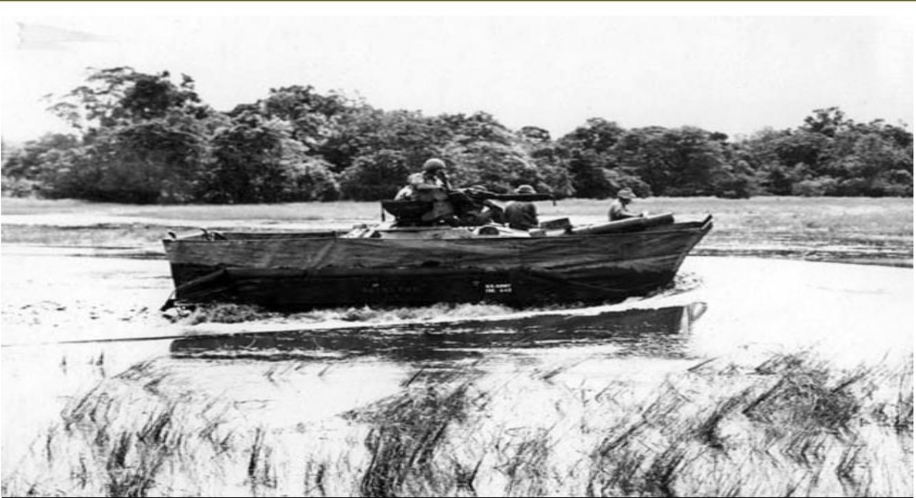
Scimitar with its flotation screen erected crossing a river during swimming trials. As well as the crew commander and gunner standing to provide guidance to the driver, a number of additional trials personnel have hitched a ride on the vehicle.
